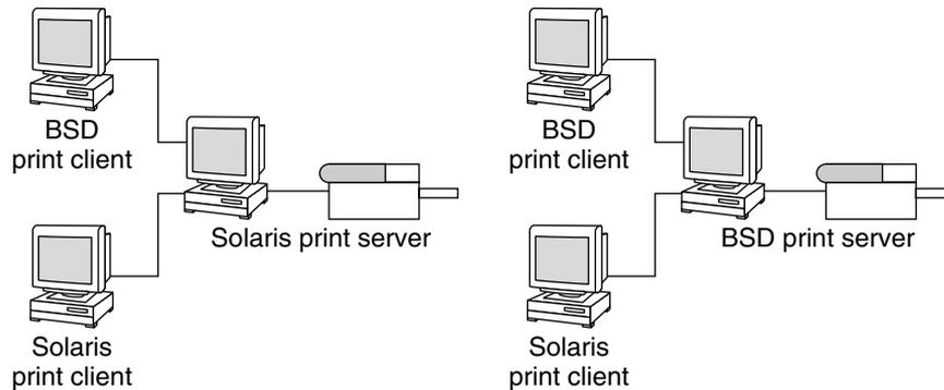
FIGURE 2-2 Solaris and lpd-Based Systems Print Configuration
